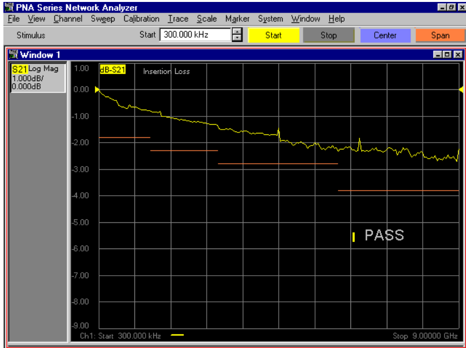
Figure 5-18 Insertion Loss Test Setup, Limit Test File Recalled
