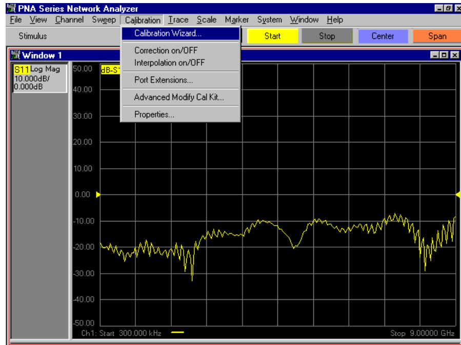
Figure 4-2 Calibration Menu on Network Analyzer
