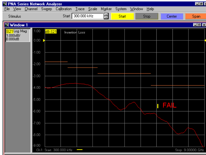
Figure 5-13 Insertion Loss Limit Test Being Run On ECal Module
